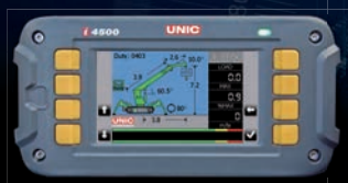
Full safe load indicator
