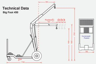
Note: Counterweights must be secured before lifting
